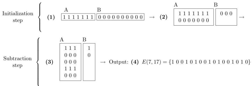
Figure 1. Euclid’s and Björklund’s algorithm to generate a maximally even rhythm with 7 “notes” (strong beats) and 17 pulses.
